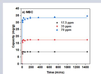
The Engineered Coal adsorbs agricultural pollutants quickly. Figure below shows that adsorption happens within the first few minutes of exposure.
