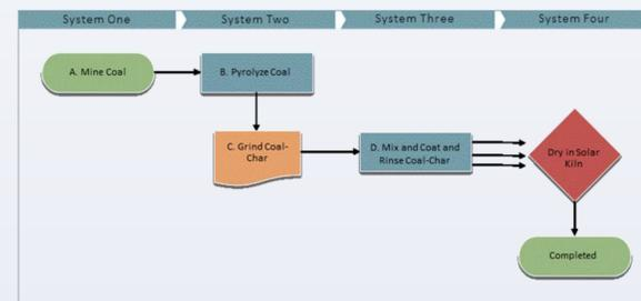
After the coal is mined, depending on the coal grade, it may be pyrolyzed in a continuous reactor (400 to 900°C with a residence time of a few seconds to a few minutes) or engineered directly. The coal is ground and then moved to the mixer and mixed while spraying with a salt solution until slurred. The salted coal-char is then transported to the solar hybrid kiln for drying. This process is repeated two more times to produce and fix metal oxides to the coal surface.
